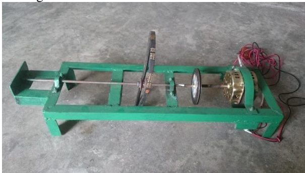
Fig 6: Constructed electromagnetic braking clutch
